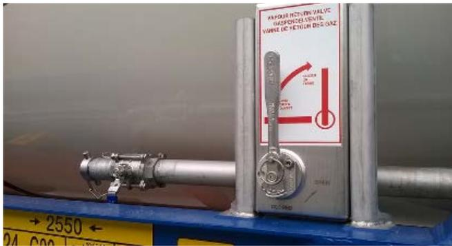
1.5 Bottom control of the top closure airline valve and airline extended to the bottom side rail
