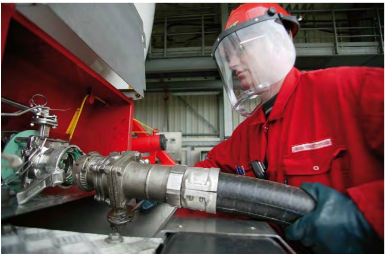
Connecting a discharge hose to the tank container bottom valve
