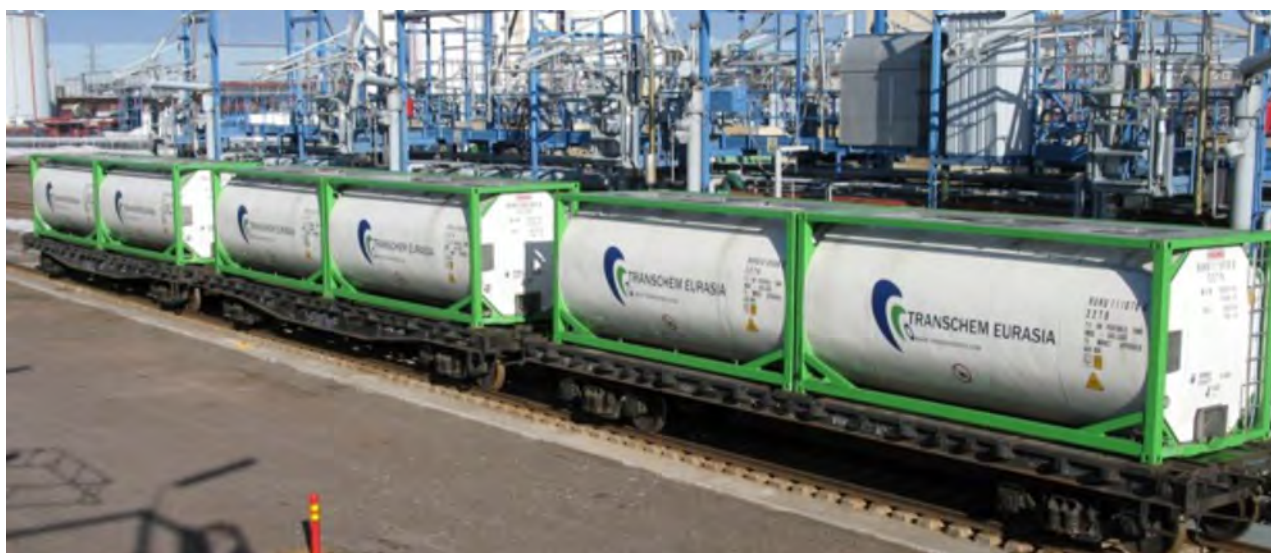
Tank containers are intermodal and used for transport of liquids and liquified gases by road, rail and sea. The photograph shows a consignment of standard liquid tank containers at a rail terminal and waiting for the cargo to be discharged directly to the chemical facility
